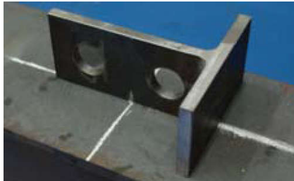
Figure 6 - T-Perfobond connector (Vianna, 2009).
