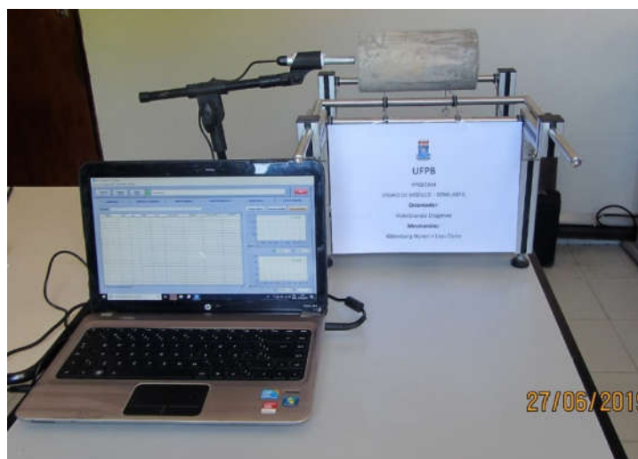
Figure 18 - Sonelastic® test setup
