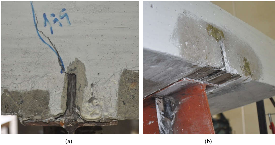
Figure 30 - Post-peak configuration of connection region for specimen with ribbed slab (a) and solid slab (b).
