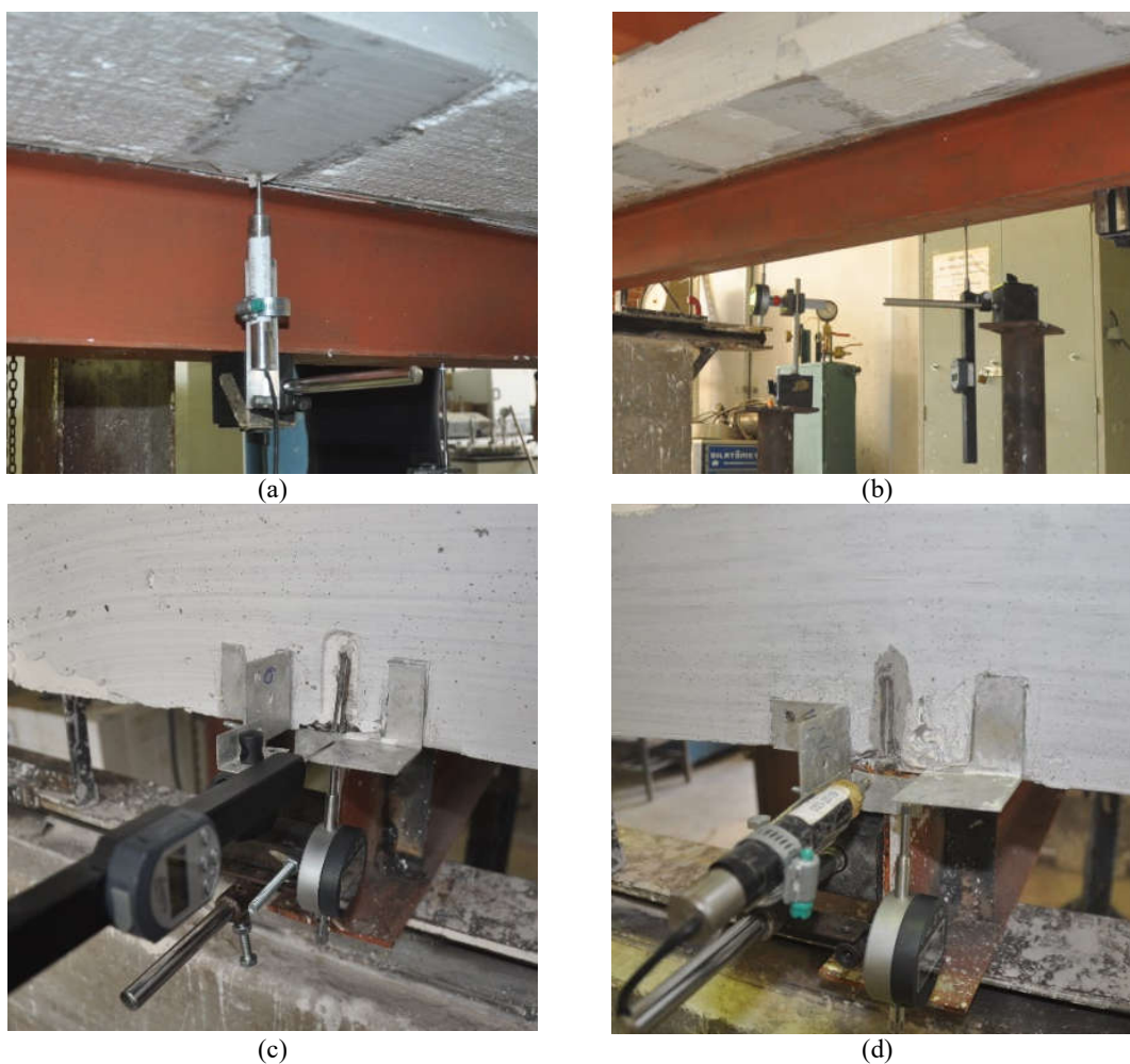
Figure 22 - Measurer device positions. Uplift at mid-span (a); Third-span and mid-span vertical displacement (b); Slip and uplift at supports (c) (d).
