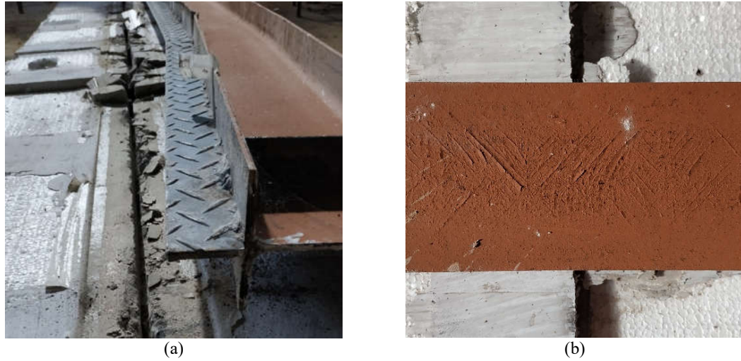
Figure 31 – Configuration of beam and connector after the flexural test. (a) demolished composite beam; (b) detachment of protective paint on the bottom flange.
