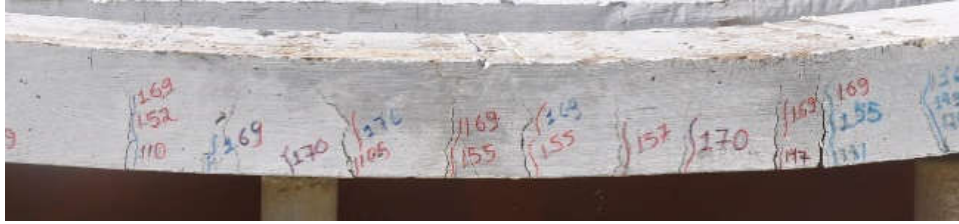
Figure 27 - solid slab cracking
