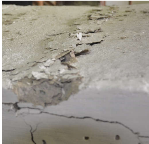
Figure 28 - Crushing of concrete slab in MAC slabs.
