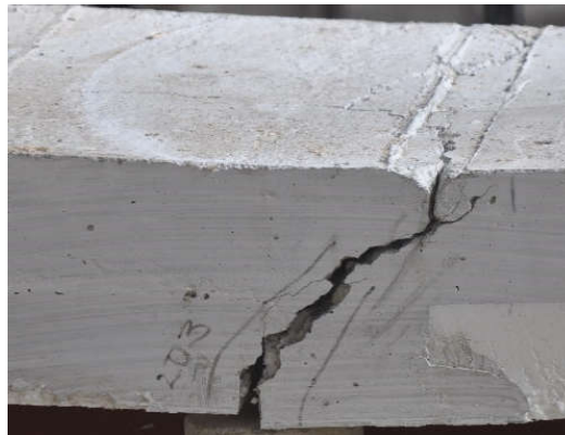
Figure 29 –Ribbed slab Cracking.
