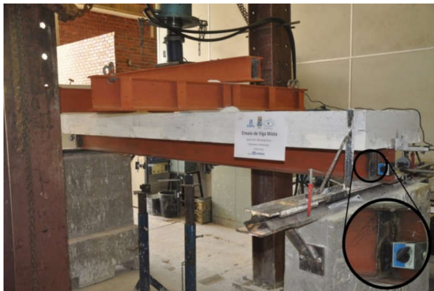
Figure 21 – Overview of Flexural test setup with detail of the web stiffener.
