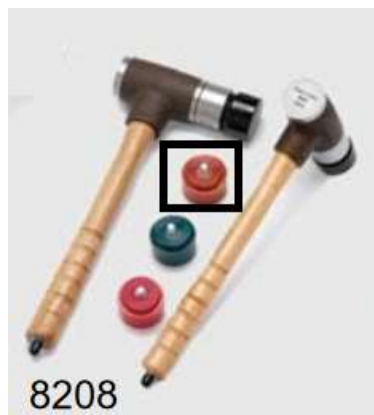
Figure 4 – Impact hammer used on tests highlighting the tip used. (Source: Product brochure, modified)
