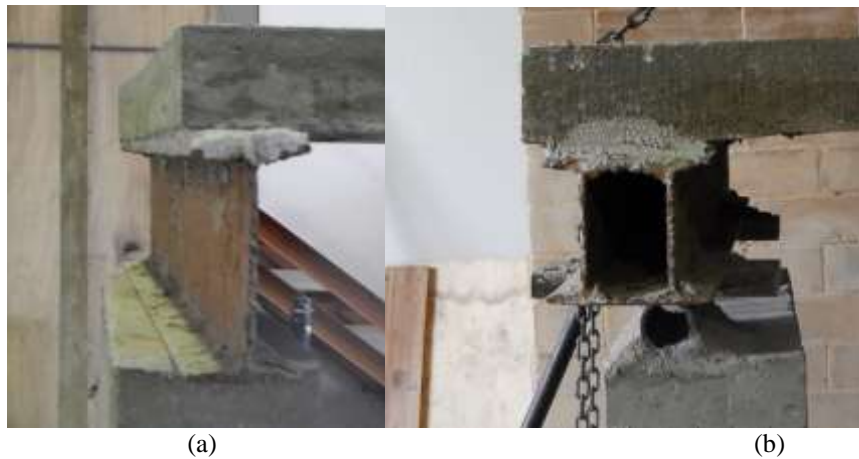
Figure 11 – Detail of continuous support line of S1 from (a) front side and (b) bottom side
