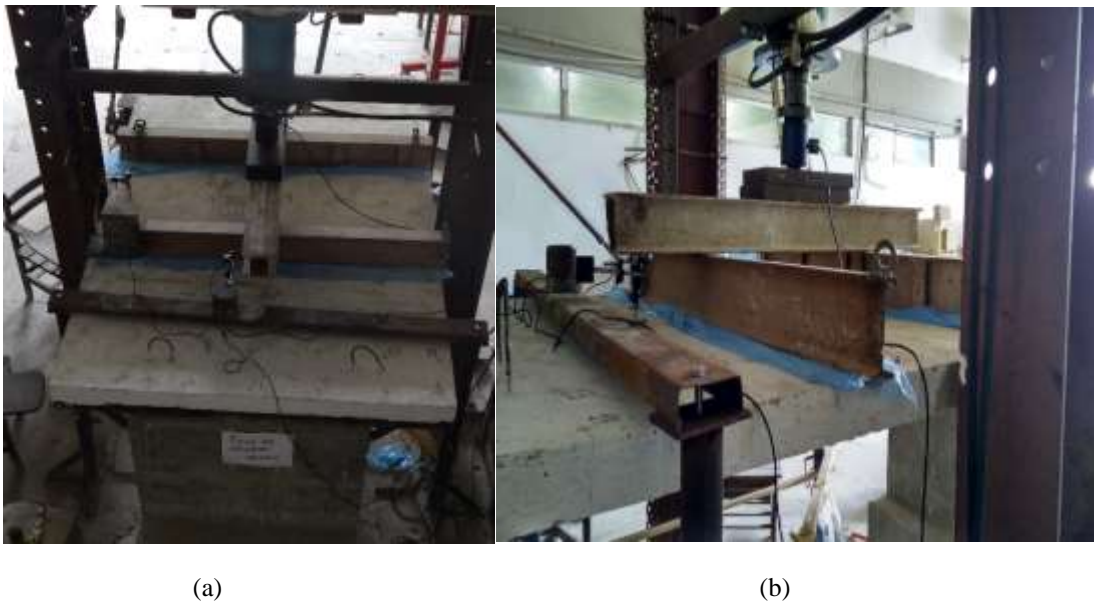
Figure 17 – Static load system to induce cracking in S2 (a) superior view and (b) side view.
