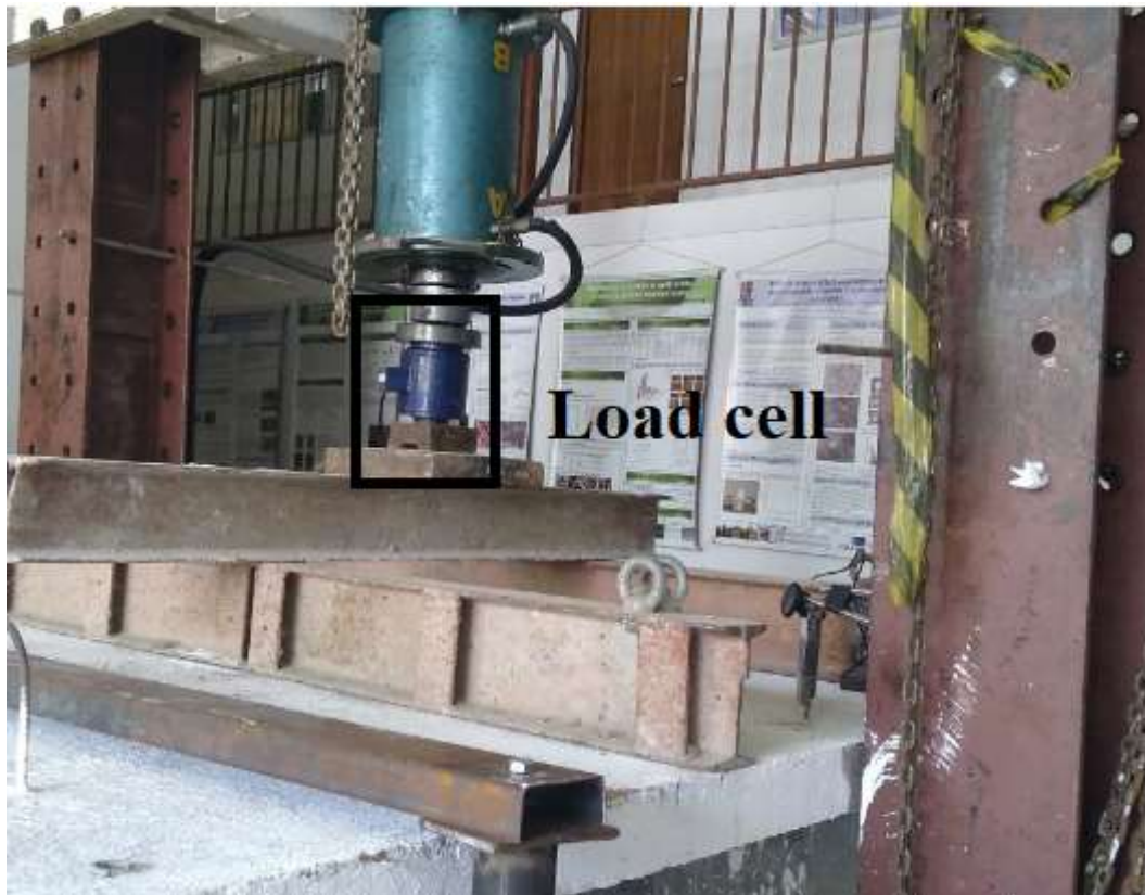
Figure 2 – Load cell used for static load application.
