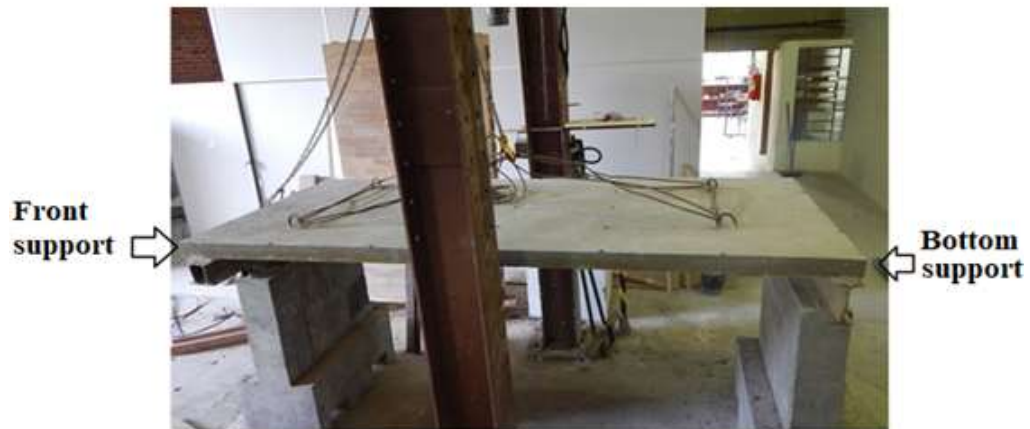
Figure 10 – Side view of S1 showing the continuous support line.
