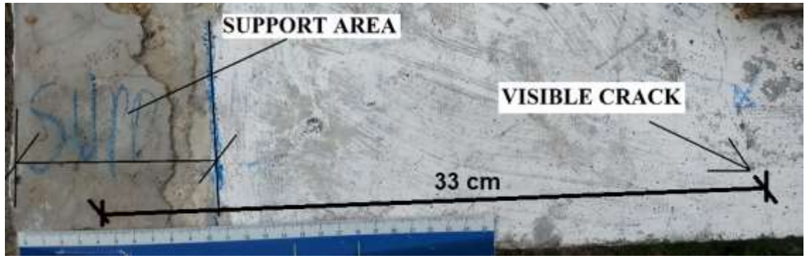
Figure 67 – Visual crack in the bottom of S2.
