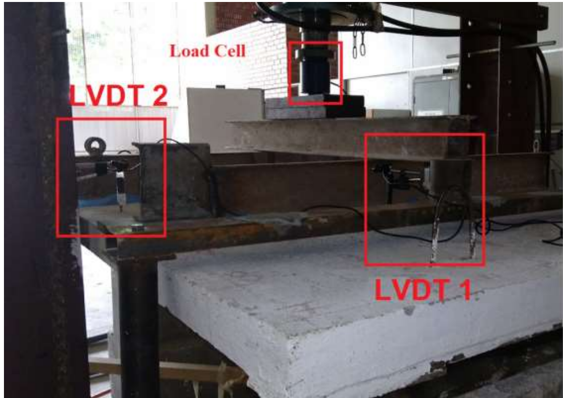
Figure 19 – LVDT used on S2 to measure deflection during static load test
