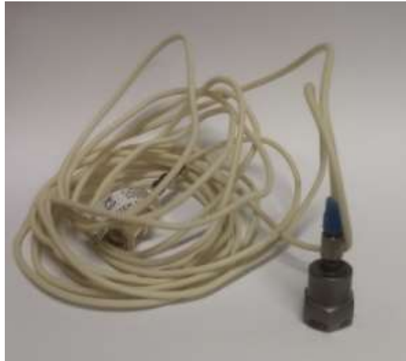
Figure 6 – Accelerometer used for testing
