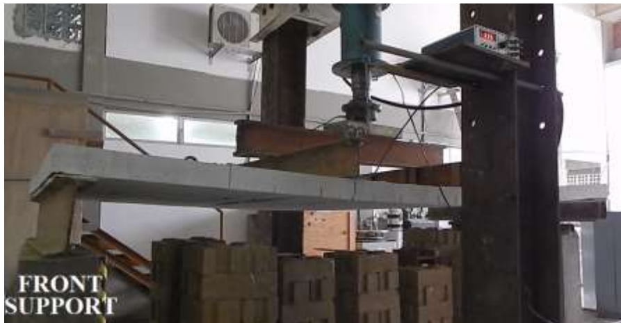
Figure 15 – Static load application in S1 (side view).
