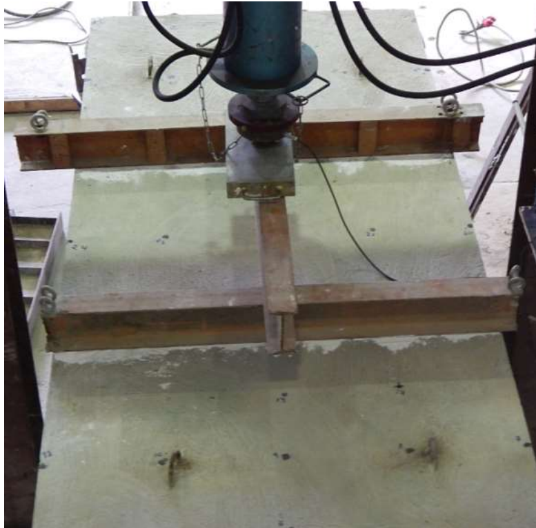
Figure 16 – Static load application in S1 (superior view).
