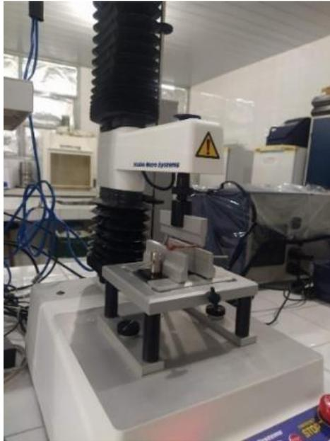
Figura 4 Texturômetro universal teste TA-XR plus Stable Micro Systems (Surrey, UK)
