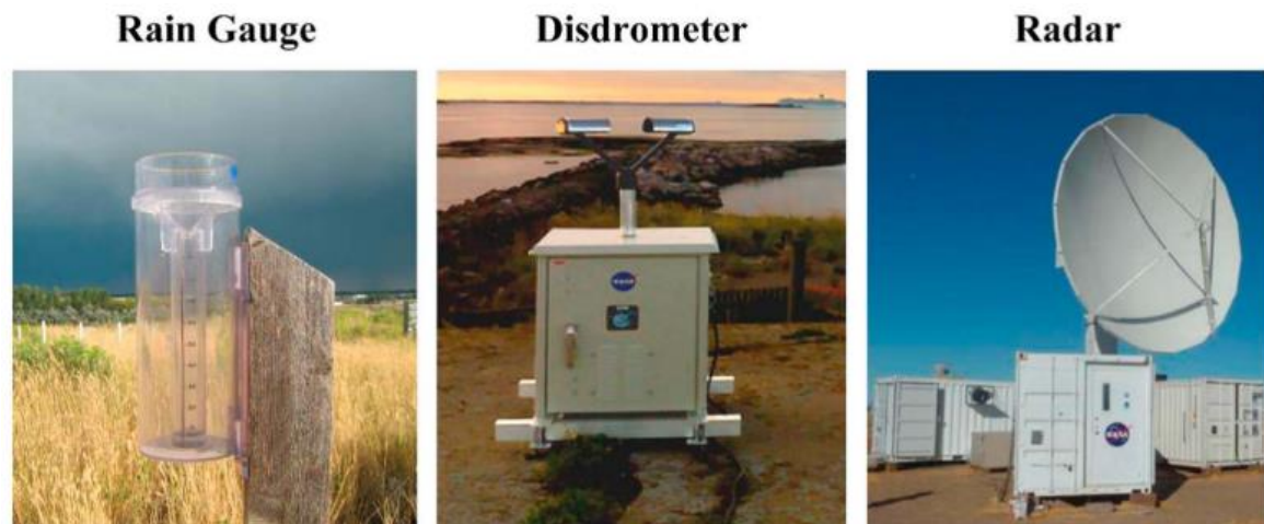
Figure 1 – Three instruments for making ground observations of precipitation. (Courtesy: Sun et al. 2018)
