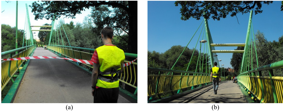
Figure 27 – Pedestrian tests: (a) Example of instrumented leading pedestrian; (b) single crossing; (Image previous used in Hawryszków et al. , 2021).
