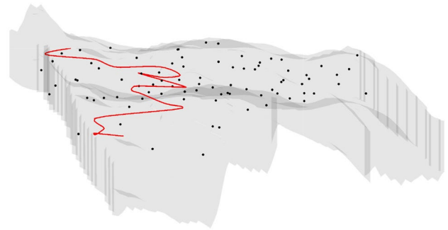
Fig. 13 3D view of selected well trajectories generated by the MILP algorithm for DP70. The paths cross flow unit targets among all possible drilling targets (black points). For the sake of visualization, the generated paths have been smoothly interpolated through the application of 3D splines over the generated paths
