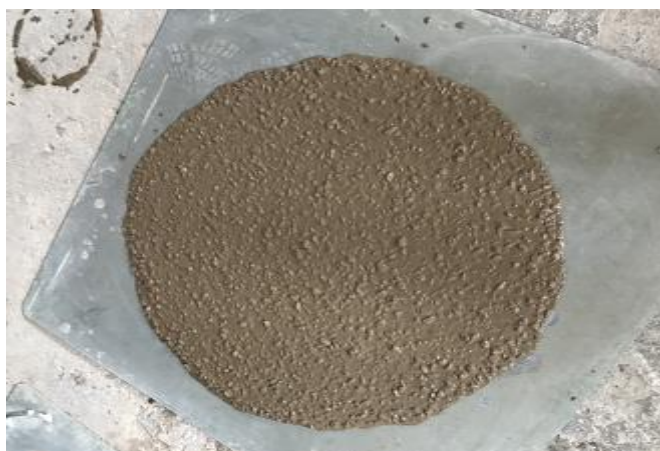
Figura 25 - Slump Flow Test
