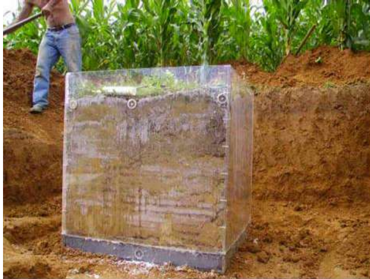
Figure 2 – Lysimeter Installation. Source: UFRGS (2004)
