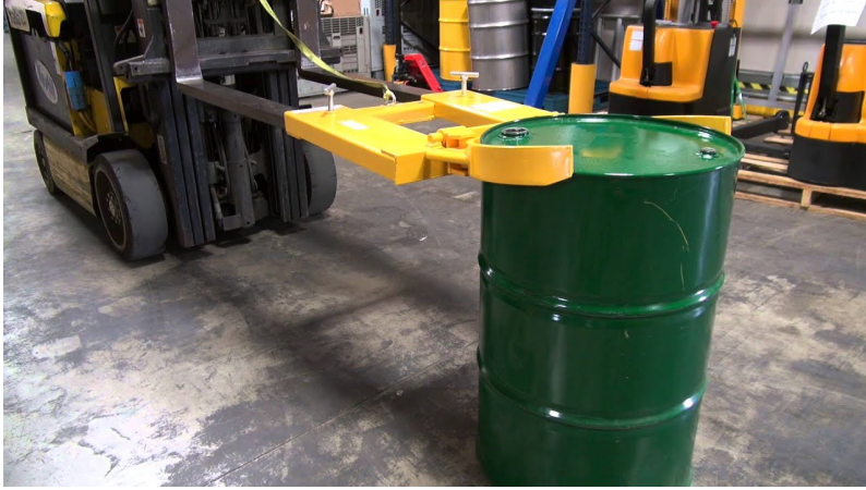
Figure 1.1: Forklift equipped with a drum clamp. Source: http://alphaliftuae.com/forklift-attachments/drum-clamp/
