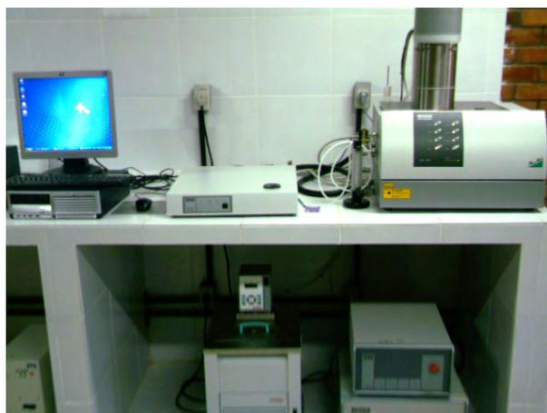
Figura 3.2 - Netzsch Microflash LFA 457 operando no LAMET
