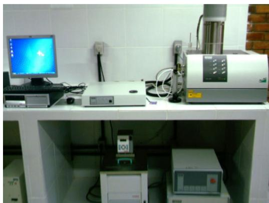
Figura 5.2 - Netzsch Microflash LFA 457 operando no LAT
