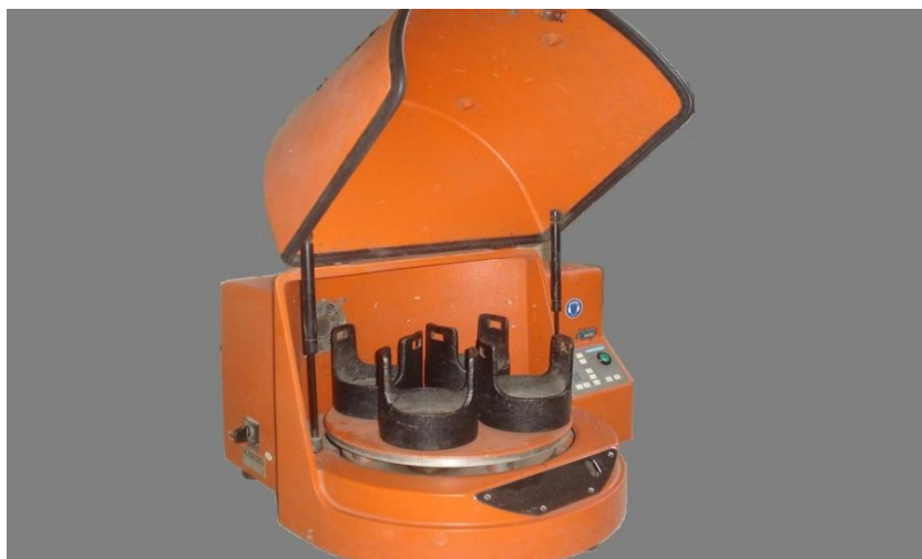
Figura 2.1 – Moinho Fritsch Pulverisette P5 .
