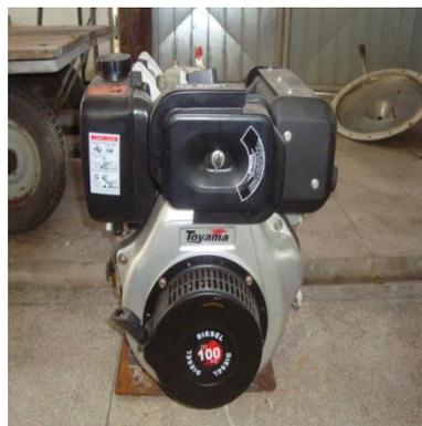
Figura AII. 4: Motor Toyama 10hp, modelo TD100FE.
